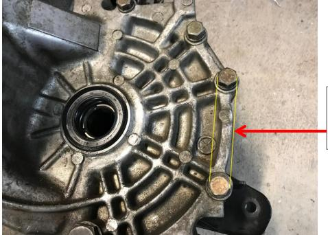
Wire placed between these two bolts to the right of drain plug.
